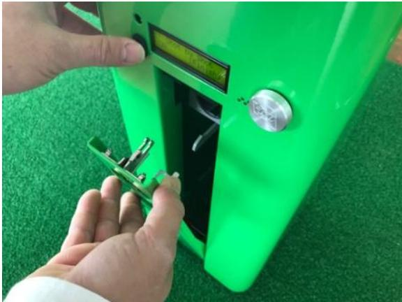
Take the ball out and set the device with the open arm so that the ball opening in the arm is centered over the tee. Then let the arm go back into the casing, the device is now aligned for the operation on the tee.
