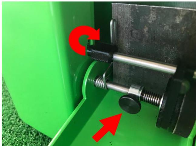
You can also adjust the backswing speed of the arm at the screw (Red Arrow). Solve the screw with your hand. To the right, the spring effect becomes stronger and so the backswing speed slower. To the left, the spring effect is less and so the arm speed will be faster.
